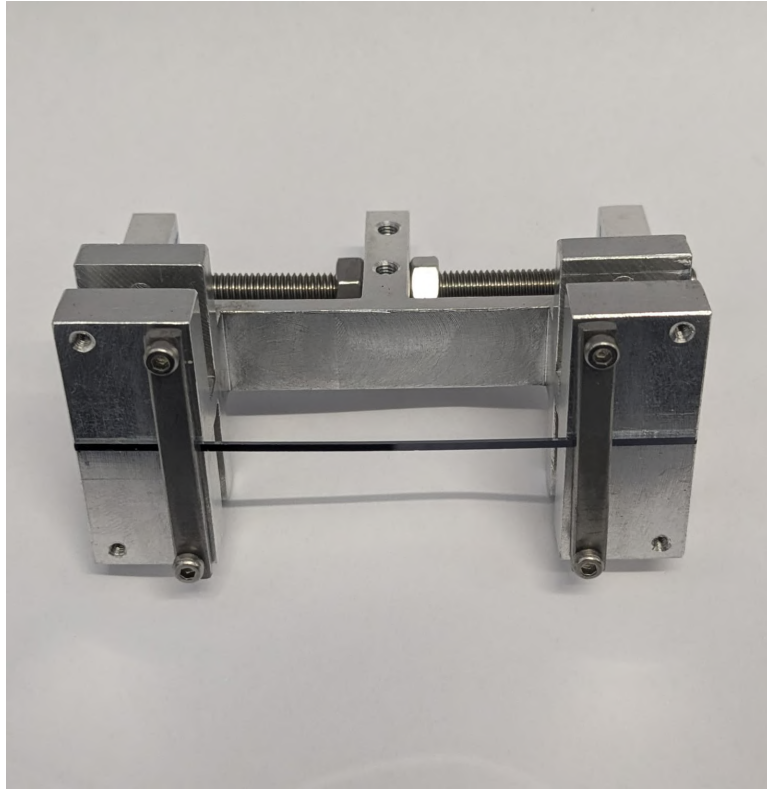
Figure 2.7: Strip crystal mounted on its holder.
