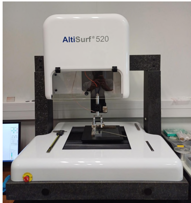
Figure 1.10: AltiSurf 520 optical surface profilometer used for the characterization of silicon crystal surfaces.
