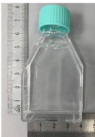
Figure 2.4: Example of a plastic flask. The cells are deposited on the front face which consists of a 1.5 mm-thick polystyrene layer. The area of the deposition is  $12 \text{ cm}^2$ .
