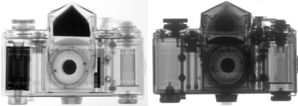
**Figure 2.** Example of a neutron imaging (left) of an analog camera in comparison with X-ray imaging (right), where neutrons make it possible to see not only heavier materials such as metals, but also some light materials such as hydrogenous substances, plastics etc. (Figure adapted from PSI website (see the link in the references)).
