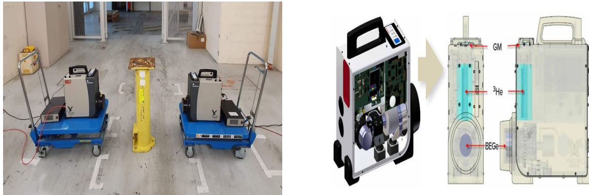
Figure 3.7: Falcon 5000 detectors with the readout electronics during acquisition in the radioanalytical laboratory at RWTCS (left). The corresponding detector layout (right). A Geiger-Muller (GM) tube is included for monitoring of the dose rate. A moderated He-3 tube is dedicated to neutron measurements (optional). BEGe Technology Germanium Detector included in HPGe Falcon 5000 enhances the efficiency and resolution at low energies, while preserving a good efficiency in high energy range [68].
