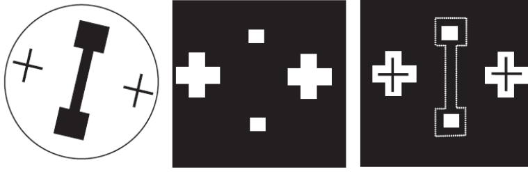
Fig. 3.4: Photomask (left) is translated and rotated below the photomask (middle) to match the alignment marks (right). Figure from [28].
