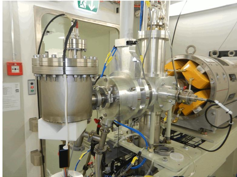
Figure 3.8 – High-sensitivity Faraday cup installed at the end of the BTL for low current performance studies.
