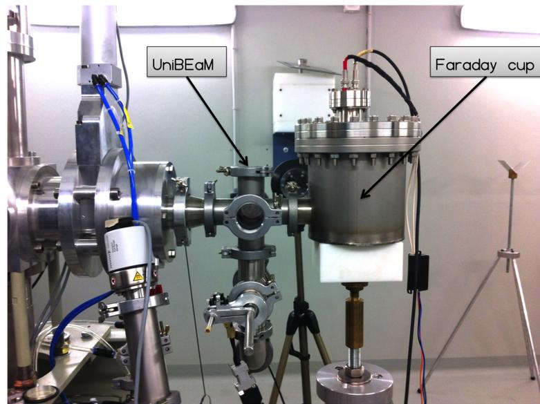
Figure 4.3 – The UniBEaM detector and the Faraday cup installed on the BTL of the Bern cyclotron.
