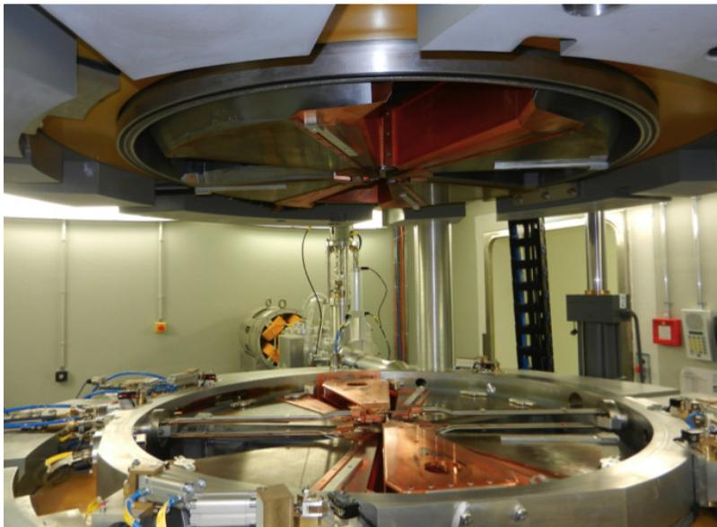
**Figure 1.** The Bern cyclotron opened during maintenance.
