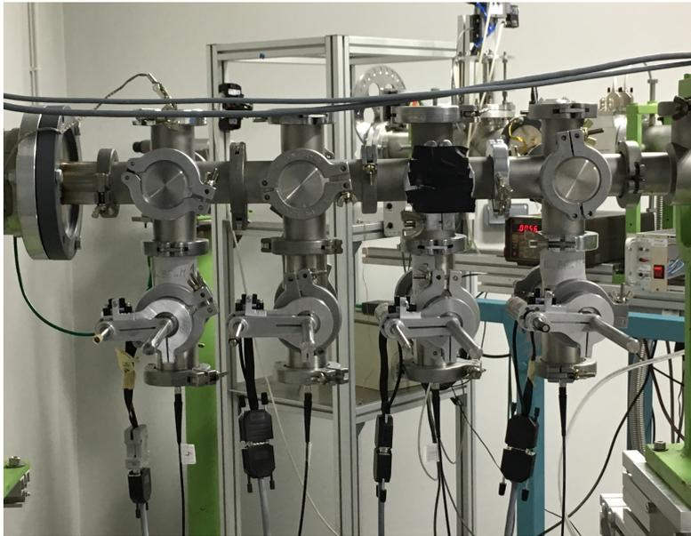
Figure 4.17 – The <sup>4</sup>PrOBεaM system for online measurement of the transverse beam emittance.
