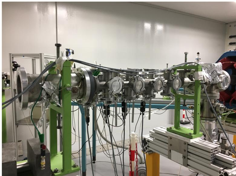
Figure 5.16 – The  $^4\text{PrOBaM}$  system installed on the beamline of the TR24 cyclotron in Strasbourg.
