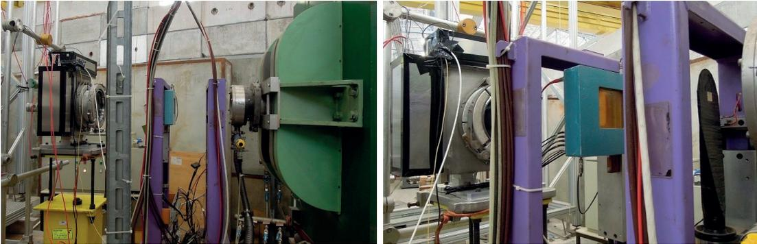
Figure 7.15 – Upstream vacuum tank, installed close to a DWC and a Scintillator Paddle.
