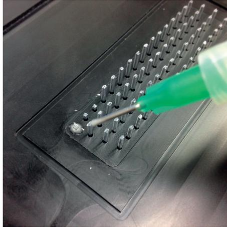
Figure 5.5 – Fibres being glued on the fibre connector.
