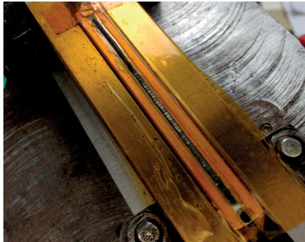
Figure 5.7 – Fibres on the mirror holder during polishing with sandpaper. *Note: there are metallic accessories on the sides of the holder in order to guarantee mechanical stability during the polishing. The orange tape helps avoiding the creation of metallic dust that could harm the fibres.*
