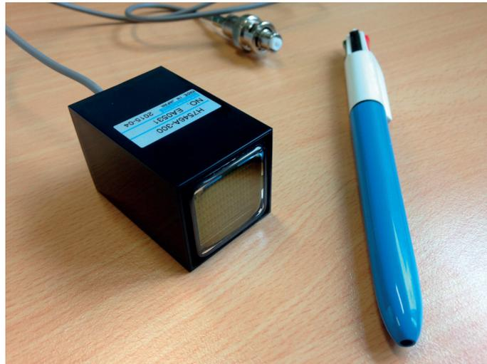
Figure 4.2 – Multi-Anode Photomultiplier H7546 from Hamamatsu.
