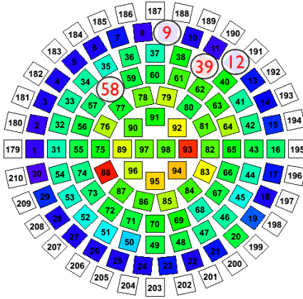
Figure 5.2: Simulated light pattern for the top PMT array, with indicated not working channels.
