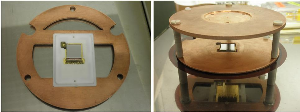
Fig. B.1: Pictures of the drift structure together with the InGrid readout installed inside the NEXT-0-MM chamber. Left: InGrid readout on a copper circular structure used as support. Right: Drift field cage together the InGrid readout. The image shows a drift with 3 cm of distance, however, most of the measurements were performed for a drift distance of 1 cm.
