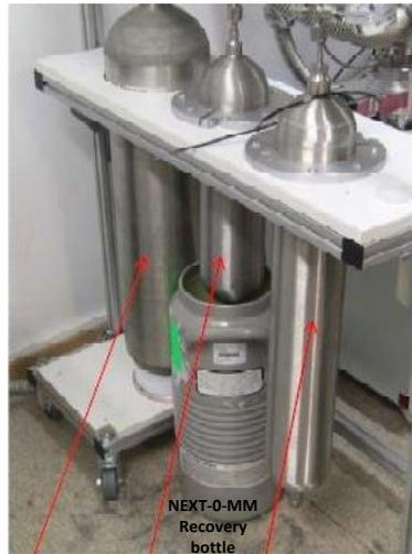
Fig. 2.4: Picture of the recovery system used to store the Xe. At the beginning, only one sample bottle was installed, recently two more bottles were added allowing to work at 10 bar in the medium size chamber.
