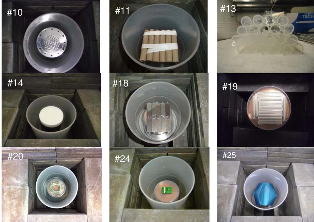
Fig. A.3: Selection of pictures of some the samples screened with the germanium detector in LSC. Identifying numbers used in Tables 2-4 are indicated.
