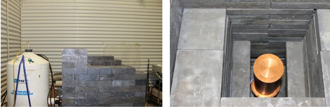
Fig. 1.10: The germanium detector used for material screening, encapsulated in a copper cryostat and inside its lead shielding at LSC.
