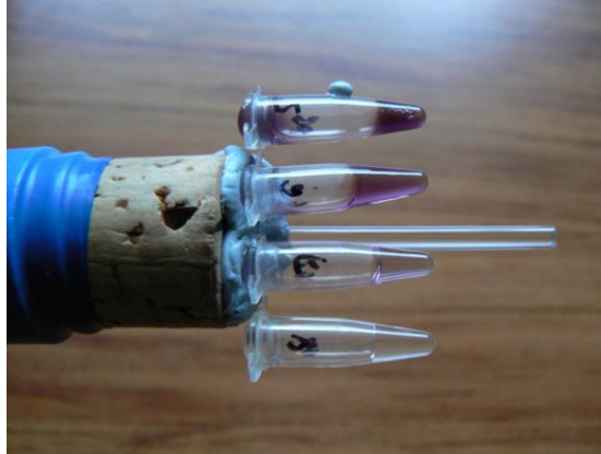
Figure 5.14 Four out of eight vials of different concentrations of gold nanoparticles were scanned at a time with multiple camera positions to cover the complete sample height.
