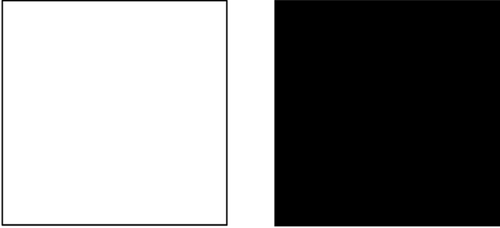
Figure 4.2 Left : An image of Si Medipix2-MXR by masking all ASIC pixels to read 1. Digitally dead pixels are shown as black (0). No pixel is observed to be digitally dead. Right : Same chip now reading 0.
