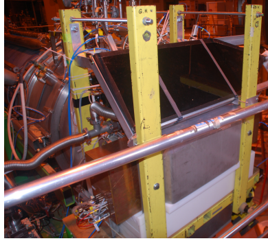
Figure 8.9: 2012 sunset final installation (see the Faraday cages backs with the electronic connections) showing the cosmic muon veto (plastic scintillator) over the shielding. The veto is mounted in 50^\circ because of space availability with present vacuum system.
