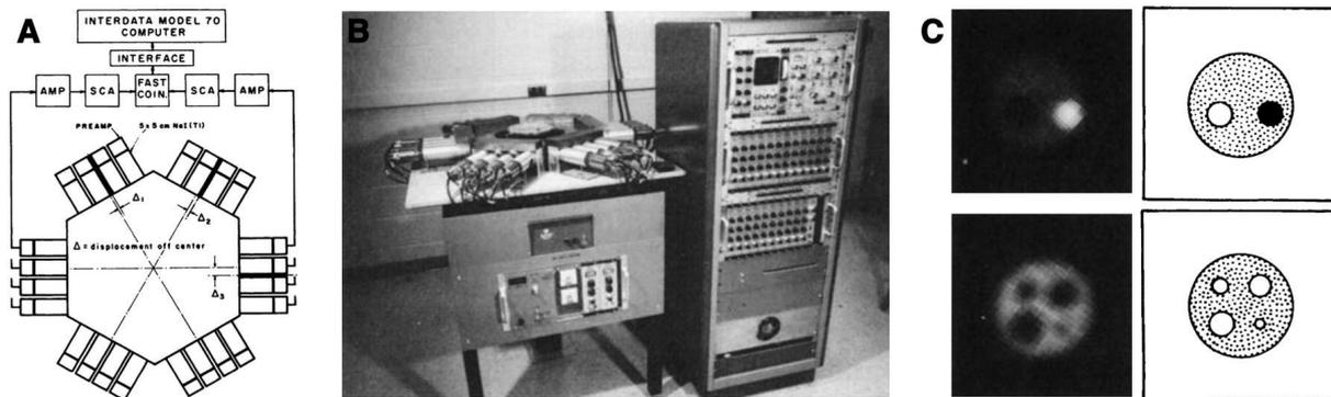
Fig. 2. First prototype of a PET detection system (A and B) based on 24 detectors consisting of single NaI:Tl scintillators coupled to single photomultipliers [2]. The images of a radioactive phantom acquired by the system are also presented (C).
