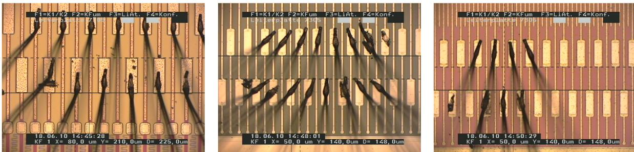
Figure 11.1: Microscope pictures of the investigated strip sensors. From left to right: CG1017, PSI02, PSI1mm. For every second strip of the PSI1mm sample the bond pad is located at the other end of the strip metalization.
