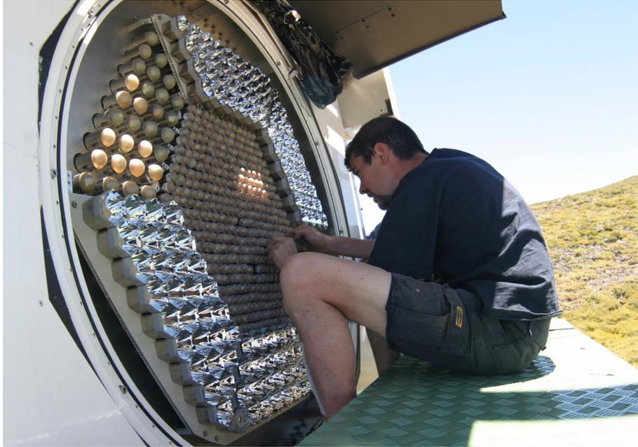
Figure 4.8: Photograph of the camera of the MAGIC telescope with opened lids while the Winston cones are being installed. The inner part of the camera consists of 397 PMTs of 1" that are surrounded by 180 PMTs of 1.5" diameter.
