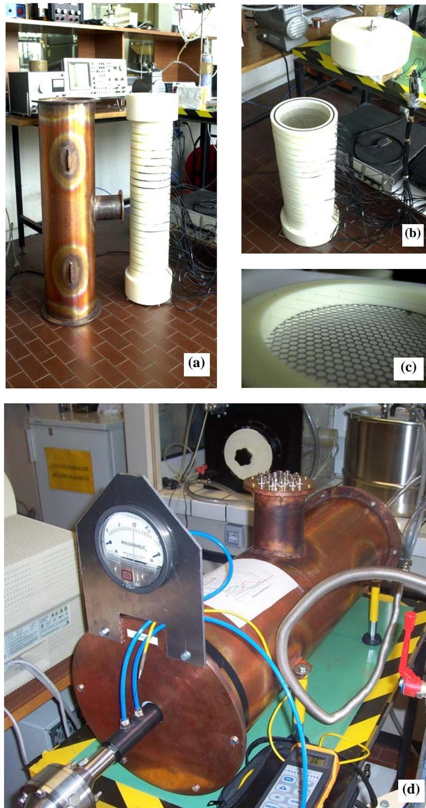
**Figure 2:** Some photos of the MCPC under construction : (a) the copper container and 20 assembled elements; (b) top view of the assembled cells and the upper end-cap; (c) single cell structure; (d) the MCPC during laboratory tests.
