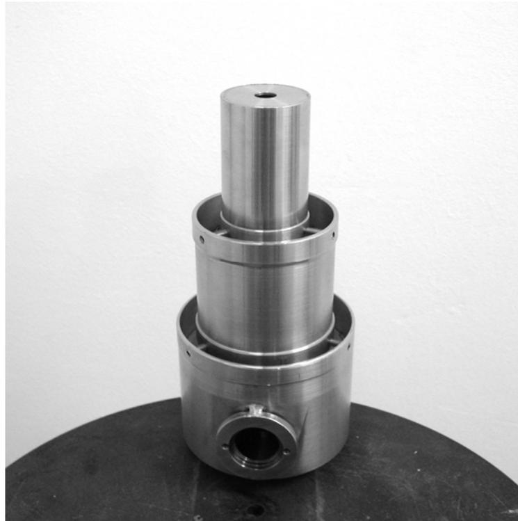
**Fig. 6.1.** *A photograph of the new expansion chamber. Note, in the lower stage, the laser beam inlet port, on which a quartz window will be mounted, and, in the upper stage, the extraction hole, 1 cm in diameter.*
