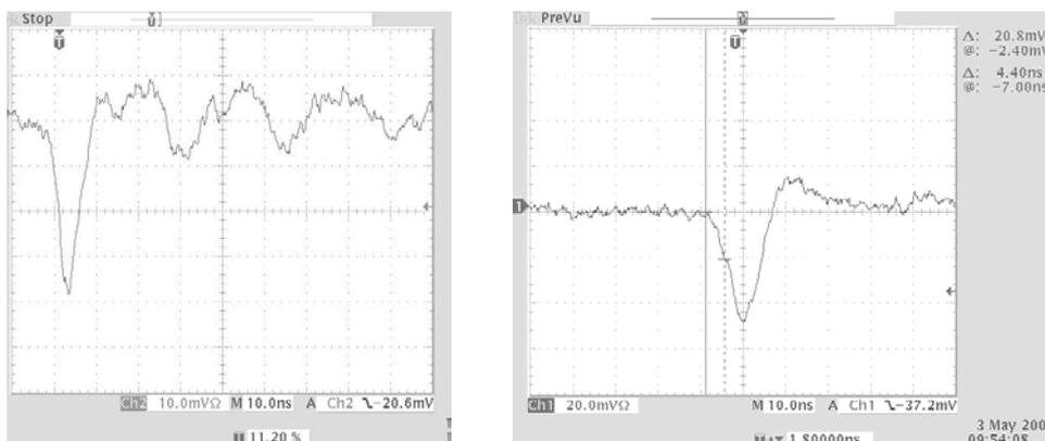
Figure 28: A fast single-photon pulse. Left: 5ns rise-time, measured in double-THGEM#4 in 1 Torr isobutane at gain  $\sim 6 \cdot 10^5$ . Right: 8ns rise-time, measured in double-THGEM#7 in 740 Torr Ar/CH<sub>4</sub> (95:5) at gain  $> 10^6$ .
