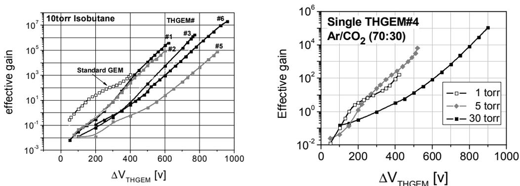
Figures 20-27: Absolute effective gain results at low pressure Isobutane and Ar/CO<sub>2</sub> (70:30) at different THGEM geometries according to table 1. The highest gains were measured on THGEM#6.
