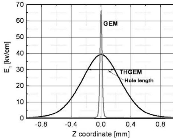
Figure 16: MAXWELL software calculation results of the electric field strength along the central axis of a standard GEM and a THGEM hole, for maximal operation voltages in Ar/CO<sub>2</sub> (70:30). THGEM#9:  $\Delta V_{\text{THGEM}}=2\text{kV}$ ; Standard GEM:  $\Delta V_{\text{GEM}}=0.5\text{kV}$ .
