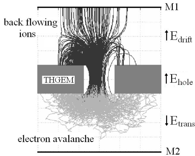
*Figure 14: The experimental setup for the ion back flow measurements in a semitransparent mode, and the simulated path of the electron and ions. The current was measured simultaneously on the THGEM bottom, on the THGEM top and on the upper mesh M1.*
