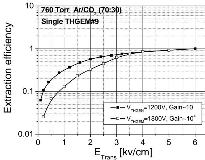
Figure 35: Electron extraction efficiency from THGEM#9 at gains of 10 and  $10^4$  in Ar/CO<sub>2</sub>(70:30), as function of  $E_{\text{trans}}$ .
