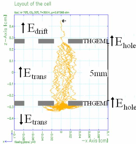
Fig.8 – GARFIELD simulation of the avalanche process in a double- THGEM #9 detector, in atmospheric pressure Ar/CO<sub>2</sub>(70:30); with  $\Delta V_{THGEM}=1350$  V, the multiplication factor of each THGEM is  $\sim 30$ , resulting in a total gain of  $\sim 900$ .
