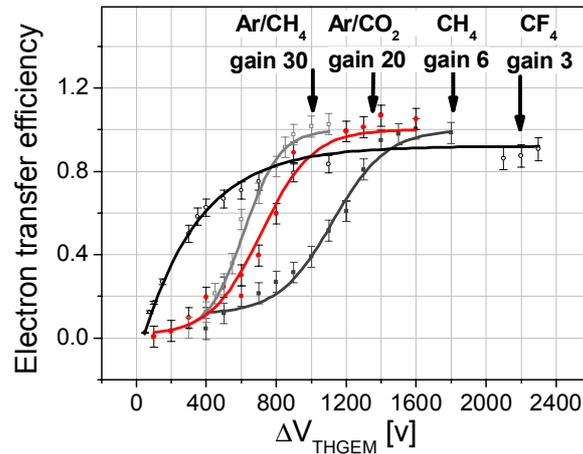
Figure 32: ETE measured with THGEM#9, as function of  $\Delta V_{\text{THGEM}}$  in a reflective photocathode mode, in various gases; full transfer efficiency was achieved at significantly lower gain compared to the standard GEM [33].
