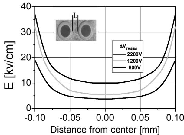
Figure 19: Maxwell calculations of the electric field on THGEM#9 top surface,  $E_s$ , along the axis interconnecting two hole centers. The electric field magnitude is above 3kV/cm, even at  $\Delta V_{THGEM} = 800V$ .
