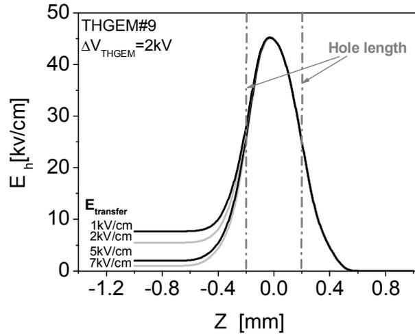
Figure 18: MAXWELL calculation results of the electric field strength  $E_h$  along the hole axis in the presence of an external field  $E_{trans}$ . A high  $E_{trans}$  applied above or below the THGEM may significantly affect  $E_h$  and the multiplication factor, outside the hole.
