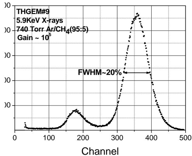
Figure 38: An energy spectrum recorded with 5.9 keV  $^{55}\text{Fe}$  X-rays in a single-THGEM#9; 740 Torr Ar/CH<sub>4</sub> (95:5), gain  $10^5$ .
