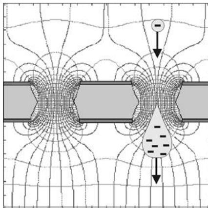
*Figure 1: Schematic view of the operational principle of the standard GEM. Electrons follow the field lines and are focused into the holes, where an avalanche multiplication process takes place at the strong electric field there.*
