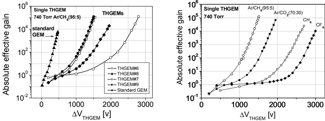
Figures 29: Absolute effective gain results at 760 Torr. Left: comparing between THGEM geometries and the standard GEM shows much higher gains at the THGEMs. Right: results of THGEM#9 at different gases in 740 Torr.
