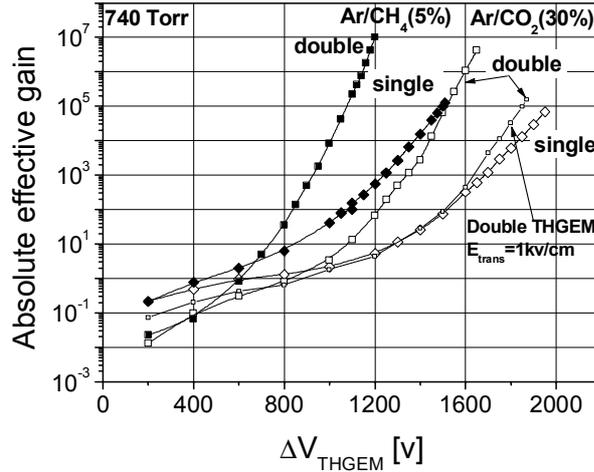
Figure 30: Absolute effective gains of single- and double-THGEM#9 multipliers, in  $Ar/CH_4$  (5%) at  $E_{trans} = 3kV/cm$  and in  $Ar/CO_2$  (30%), at  $E_{trans}$  of 1 and 3kV/cm;
