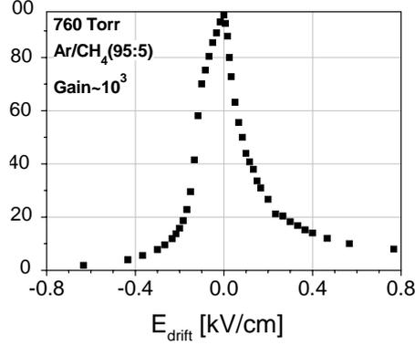
Figure 33: ETE measured with THGEM#9, as function of  $E_{drift}$  in Ar/CH<sub>4</sub> (5%); maximum ETE was obtained at  $E_{drift}=0$ .
