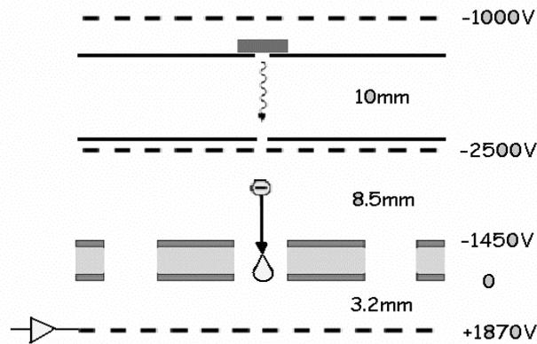
*Fig. 15: X-ray measuring scheme; the collimator focuses the beam on a small area of  $7\text{mm}^2$ ; the x-rays are absorbed in the 8.5mm gap. The electrons are focused into the holes, are multiplied and collected on an electrode below.*
