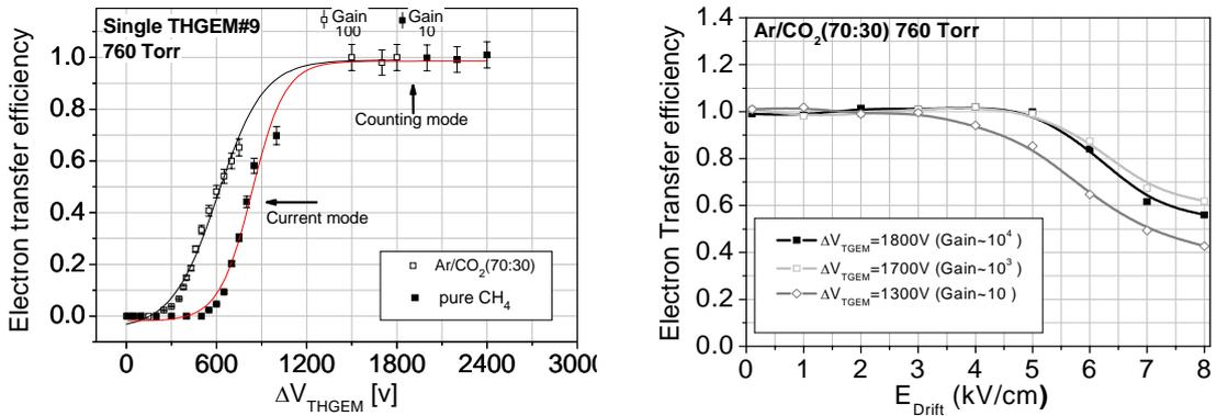
Figure 34: ETE of THGEM#9 in the semitransparent photocathode mode. Left: Inside Ar/CO<sub>2</sub> (70:30) and in pure CH<sub>4</sub>. Full ETE is reached at respective gains of 10<sup>2</sup> and 10. Right: ETE as function of  $E_{drift}$ ; Ar/CO<sub>2</sub> (70:30) at different gains.
