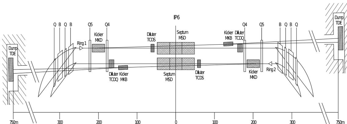
**Figure 10.1:** Schematic layout of beam dumping system elements around LHC Point 6 (distances in m).
