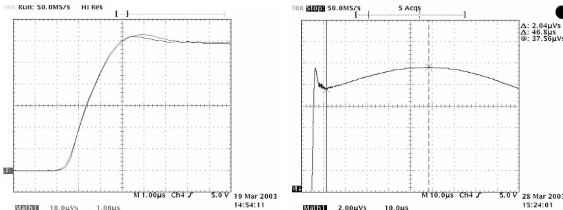
**Figure 10.2:** Start of MKD magnet current pulse at 450 GeV and 7 TeV with overshoots of 7.5% and 5.2% respectively (left); MKD magnet current pulse over 100  $\mu\text{s}$  at 7 TeV with flat top overshoot of 5.6% (right).
