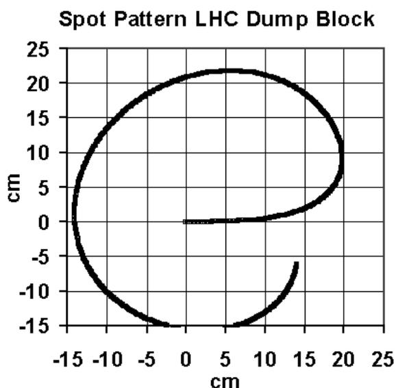
Figure 10.5: Beam spot figure on absorber block.
