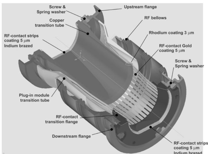
**Figure 5.3:** Details of the interconnect “plug-in module”.
