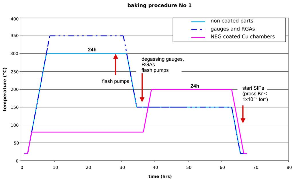
**Figure 5.7:** Proposed bakeout cycle with NEG activation.
