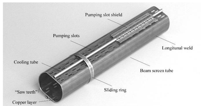
**Figure 5.1:** Conceptual design of the LHC beam screen.
