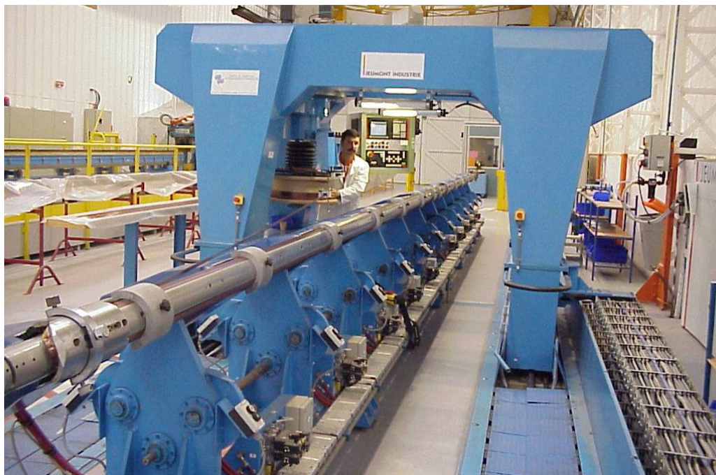
Figure 3.4: A winding machine for the superconducting coils.
