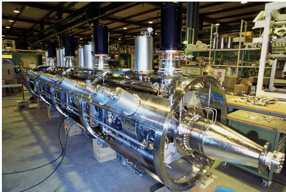
Figure 4.2: Four-cavity module during assembly.
