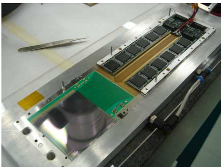
Figure 2.9: Photograph of a silicon layer during the assembly phase.
