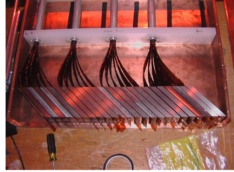
Figure 6.5: Photograph of the ZDC HAD section.
