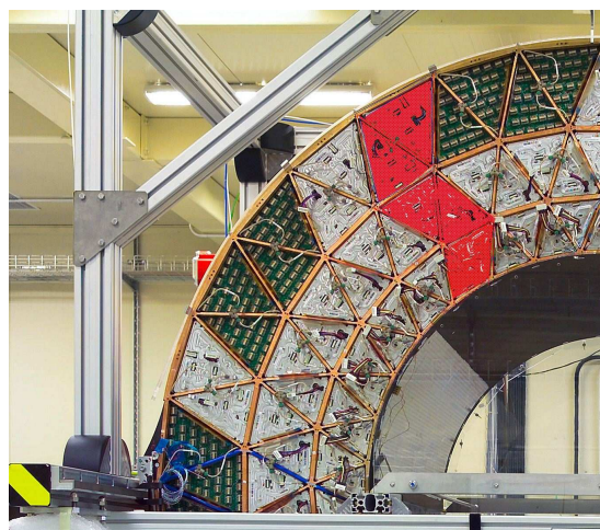
Figure 4.9: Photograph of one quarter of the barrel TRT during integration. The shapes of one outer, one middle and one inner TRT module are highlighted. The barrel support structure space-frame can be seen with its triangular sub-structure.
