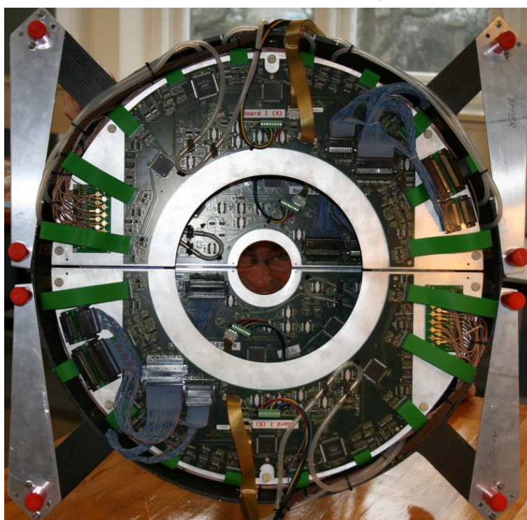
Figure 5.13: Assembled FMD3 detector. The side of the detector points away from the interaction point. Two outer digitizer boards can be seen while the two inner digitizer boards are partially covered. Each of the green cables connects a silicon module mounted on the other side of the support plate to its respective digitizer board.
