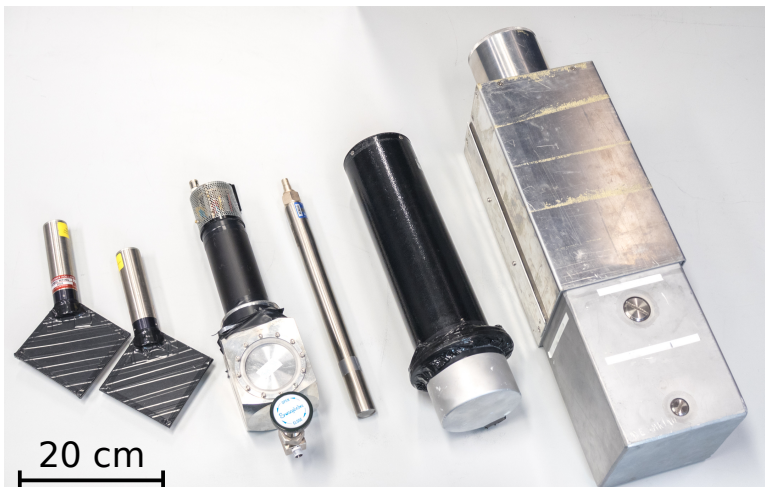
Figure 2: Example of detectors available at the STF. From the left, two plastic scintillator paddles read out by PMTs, one He-4 cell (operated at 5 atm) read out by a 2" PMT, a He-3 tube (calibrated efficiency of 96.1% at 2.5Å) and two NE213 liquid scintillator (0.43 and 4.5 l) read out by a 3" PMT.
