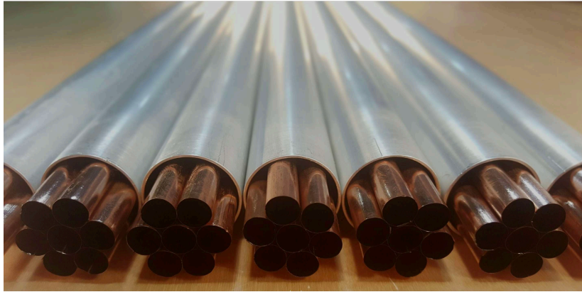
Figure 1.6: Cross-sectional view of the BCS detector from [42]. The copper straws inside the aluminium tubes are exposed.
