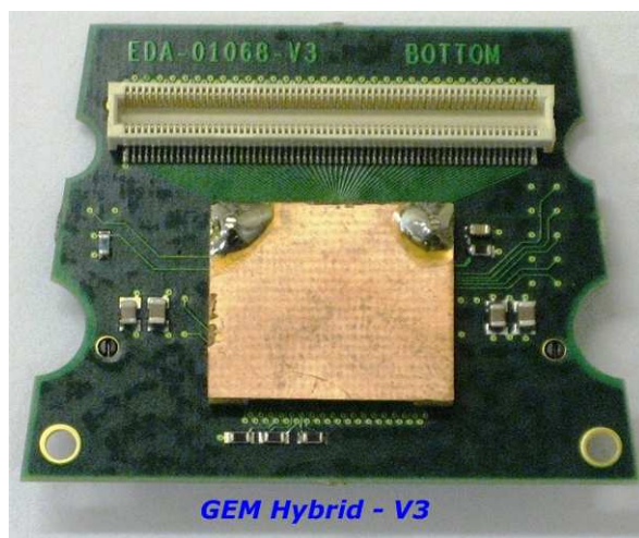
Figure 5.18: The TOTEM gas detector hybrid carrying one VFAT readout chip (under the cover).
