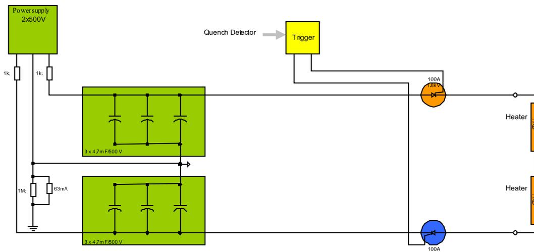
**Figure 6.7:** Quench heater power supply functional diagram.
