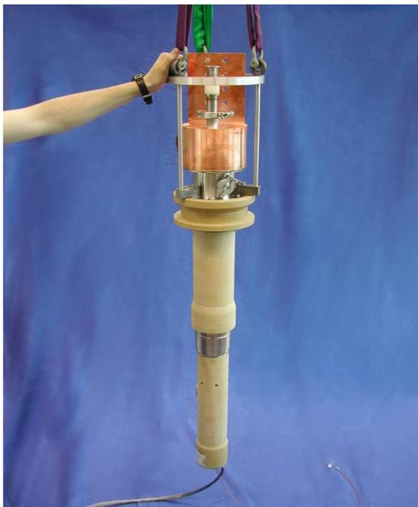
**Figure 6.5:** 13 kA CERN prototype HTS current lead.
