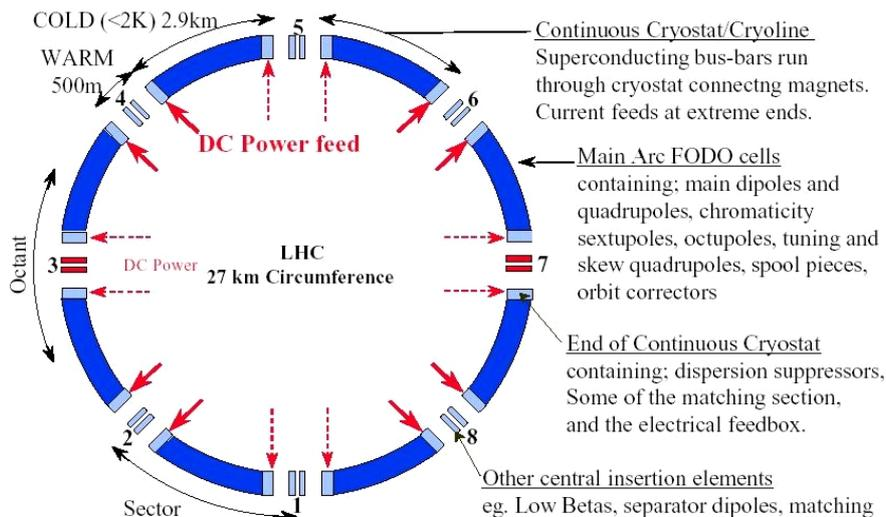
**Figure 6.2:** Powering of the eight arc cryostats.
