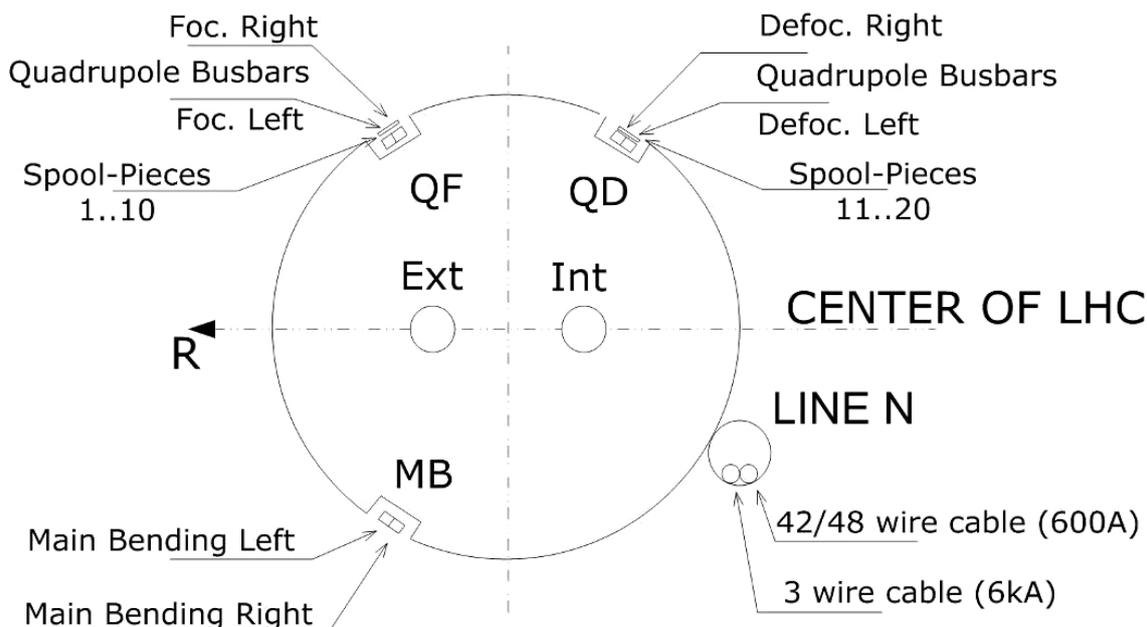
**Figure 6.3:** Cross-section of LHC arc cryo-assembly with bus-bars.
