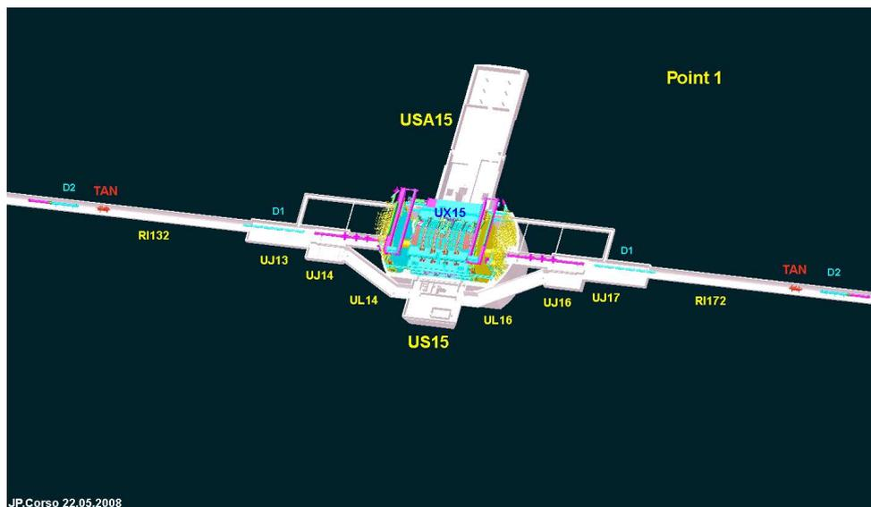
**Figure 1.2:** Geometry of the IP1 area of LHC. The structure seen in the center represents the ATLAS detector surrounding the interaction point. The straight line from top-left to bottom-right indicates the long straight section of the LHC tunnel and the LHCf detectors are installed at the places marked 'TAN' at both sides of IP1.
