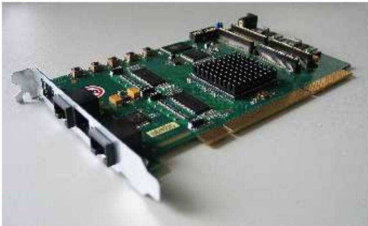
**Figure 6.8:** H-RORC data pump and FPGA coprocessor.
