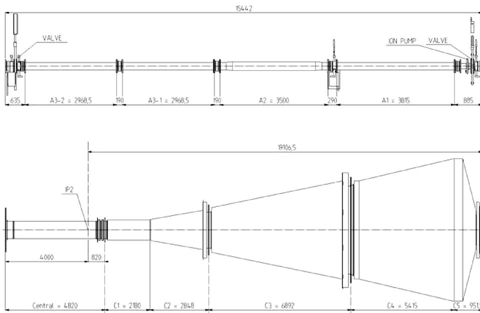
**Figure 2.3:** Layout of the ALICE vacuum chamber.
