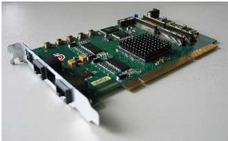
Figure 6.8: H-RORC data pump and FPGA coprocessor.
